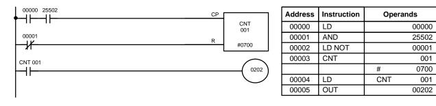
**Caution** The shorter clock pulses will not necessarily produce accurate timers because their short ON times might not be read accurately during longer cycles. In particular, the 0.02-second and 0.1-second clock pulses should not be used to create timers with CNT instructions.
